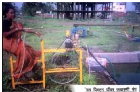
Bicycle-powered pump developed by Chandrakant Pathak.
